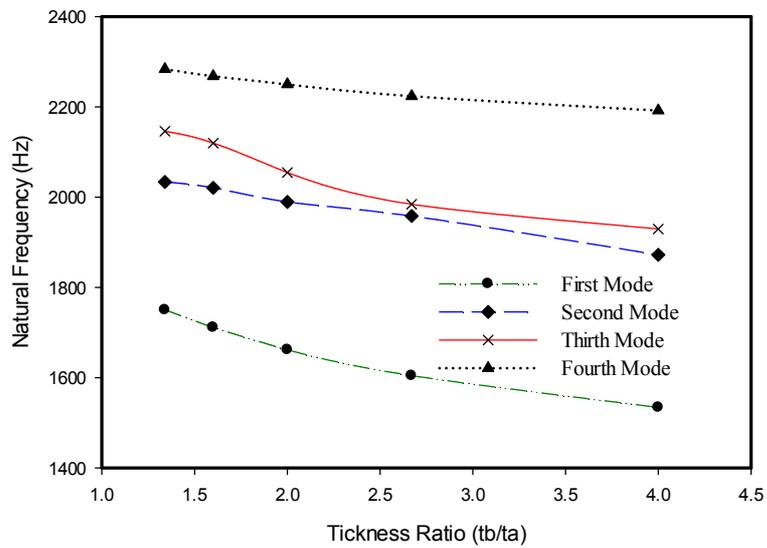
Figure 5 Natural Frequencies for First Fourth modes for Model (2).
