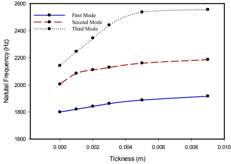
Figure 3 Natural Frequencies for First Three modes for Oblate Spheroidal Shell
