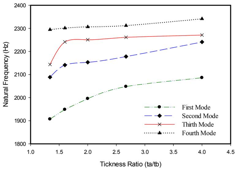
Figure 4 Natural Frequencies for First Fourth modes for Model (1).
