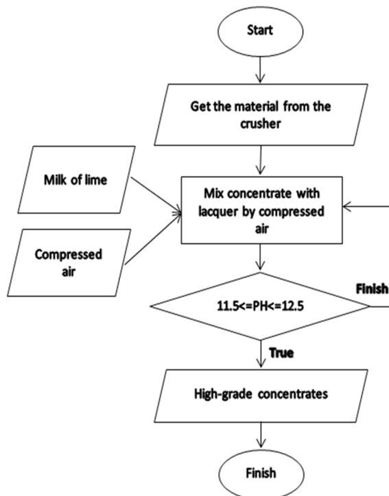
Figure 1 Copper Flotation Flowchart
